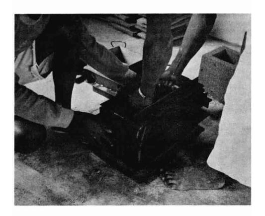
Remove core (center part of mold). Lift block to drying area. Pull out pins at opposite corners and carefully remove outside of mold.
