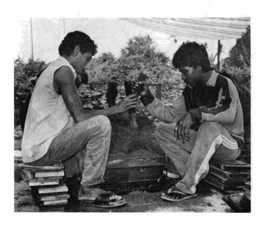
5cm each time, tamping after each addition. Do not over tamp. This will be learned with practice. Pat with side of stick and level off. Place 18mm oversized plywood on top and flip mold over to remove.
